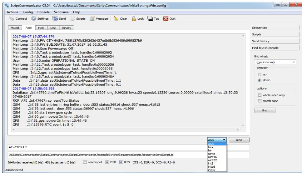
All sent and received data can be shown in a console and can be logged in an html and a text
